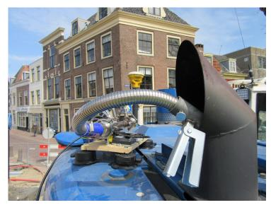
Different measurement and monitoring systems developed to screen, test, and monitor NRMM in normal use. Assisting operators with reporting and mitigation measures.
