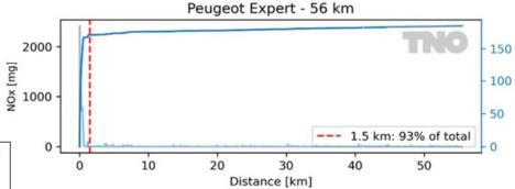
Euro-6d diesel NOx emissions, over a 56 km trip: 68%-93% during cold start
