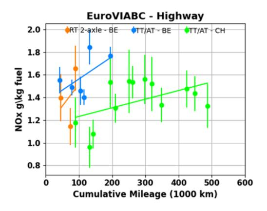
Deterioration trend **after** removal of high-emission records now "lower" 0.16 vs. 0.40 gNOx/kg fuel per 100'000 km
