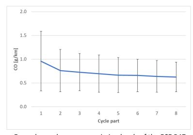
Example graph: average emission levels of the ECE R47 driving cycle second-by-second data for minicars, for CO. Error bars indicate min and max values within the test vehicles (after averaging in each vehicle's cycle runs). Parts 1-2: cold start, parts 3-8: hot.
