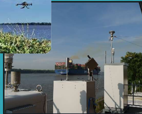
Sampling passing by vessel plumes Wedel, Sep 2020
