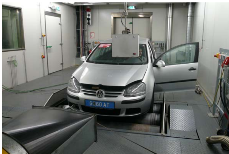
Figure 7-4: Chassis dynamometer test cell
