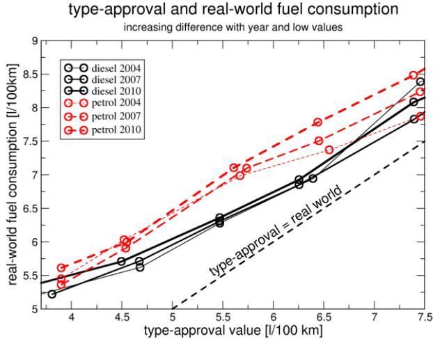
**Figure 5 Real world versus type-approval fuel consumption**
