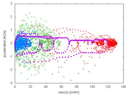
**Figure 4 Different real-world driving cycles (red +: CADC motorway; green x: CADC urban; blue \*: dutch heavy congestion) compared with the NEDC test (magenta bullets). The NEDC test has a limited variation, low accelerations, and specific constant velocities.**
