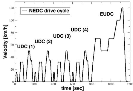
**Figure 3 The type approval test, for factory values of CO<sub>2</sub> emissions.**
