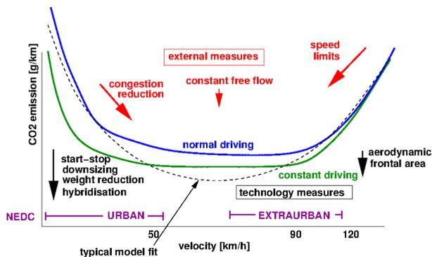
**Figure 1 The CO<sub>2</sub> emission as function of velocity alone. The regions of the NEDC test generate a focus low-velocity reduction. The typical flat minimum is not reproduced by the typical physical models fit.**
